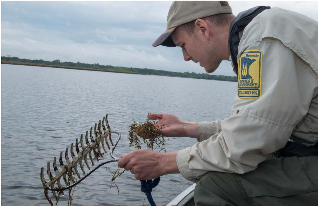
Figure 1. A two-sided metal rake for sampling aquatic plants. This sampling rake was made by welding two rake heads together. It can also be constructed by tying two rake heads together with zip ties.
