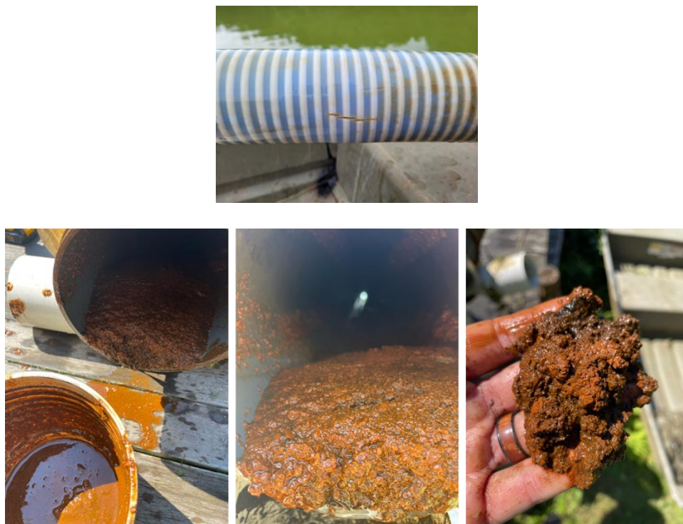
Figure 5. Cracked discharge pipe (top) and iron sludge (bottom)
