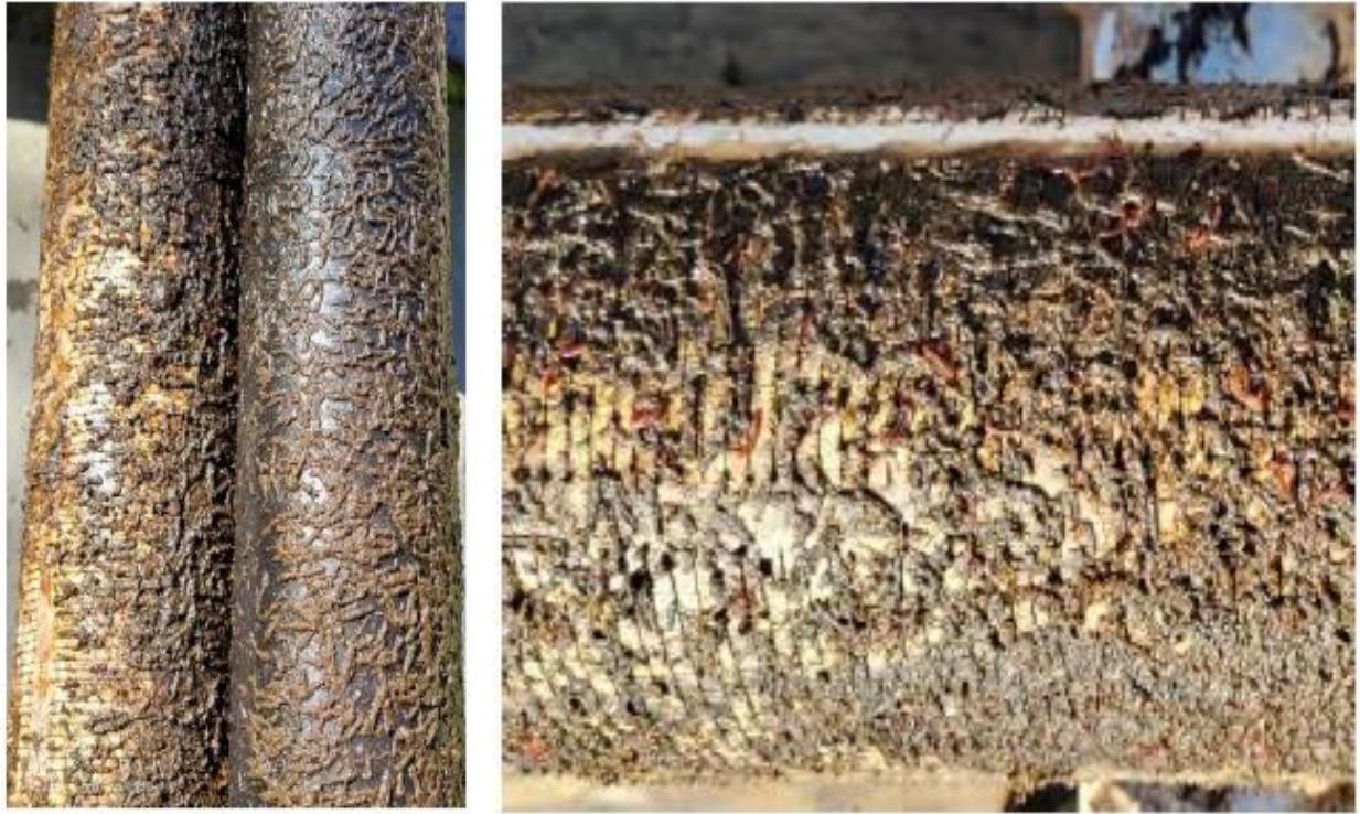
Figure 8. Biofouling of suction and discharge header pipes
